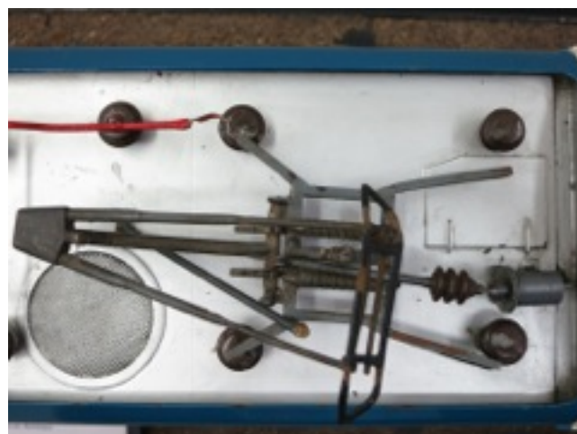
Model Locomotive, 1/24, BR class 83 2 Bo-Bo. NRM York. Surface cleaning, Pantograph Reconstruction, Replication of missing parts.
